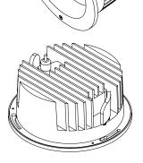
Tamperproof bezel option Necessary for 2G vibration ratings
